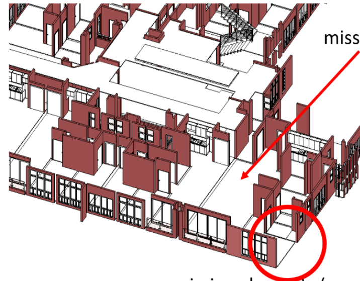
Missing elements (e.g., IfcWall) in 3D model
