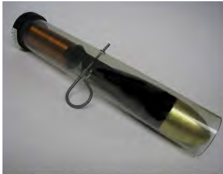
An EXpendable BathyThermograph (XBT) with it's probe inside a canister (top). On the right is an exploded view of the XBT.
